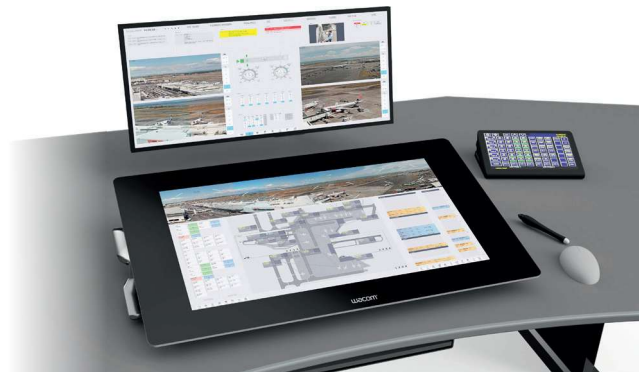
Integrated controller working position (iCWP)
